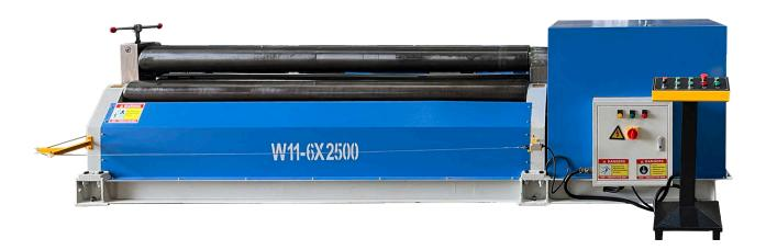
The W11 series plate rolling machine has a mechanical 3-roller symmetrical system with motorised up down movement of top idler roll which moves up and down in the centre of the two lower driven rolls.
